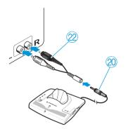
With most TVs, the RCA socket is located at the rear. If your TV has several RCA sockets, use the socket RCA output.
